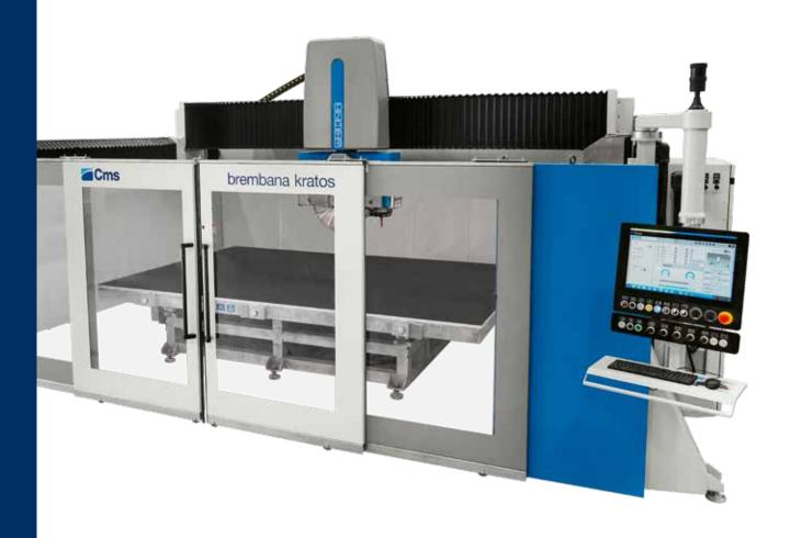
CMS brembana kratos is the ideal solution for stone fabrication workshops looking to invest in the durability and productivity of mid-size bridge saws.
