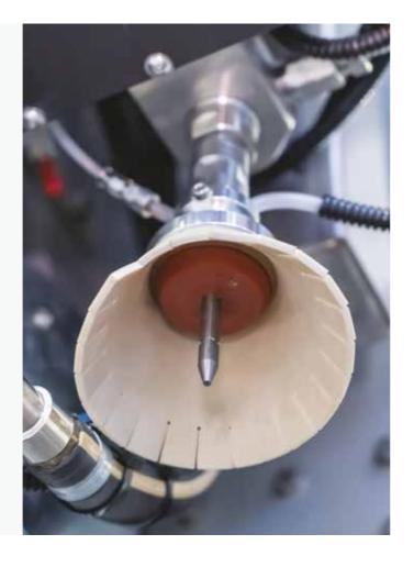
abrasive flow. If the abrasive flow is interrupted for any reason, the system will automatically stop cutting to prevent damage and scrape materials. In addition, a vacuum sensor connect to the mixing chamber constantly detect the abrasive amount and flow, providing complete real-time information on the state of wear o the cutting head.
