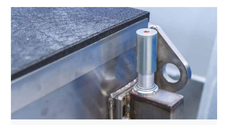
DISK PRESETTING to measure disk diameter and finger bits or core drills lenght
