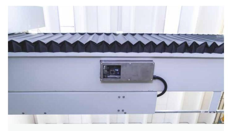
CAMERA: system to obtain the images from the working table, it permits to accellerate the pieces positioning and notice possible bugs on the slab
