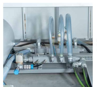
Separate double vacuum system for edge and basin forming unit with built-in tank and full proportional system
